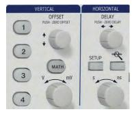
When the Math light is on, use the horizontal and vertical controls to adjust the scale and position of the Math trace.
